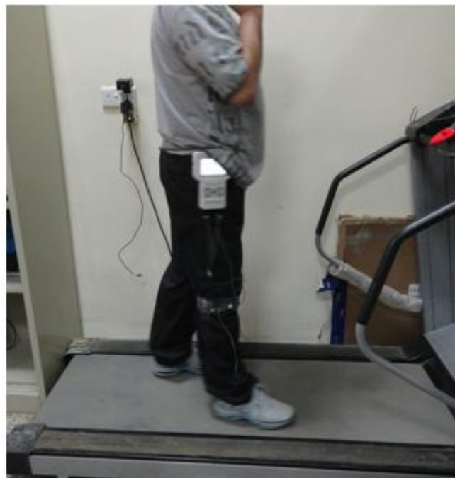
Figure. (2)The vibration measurement system using a Nor axon USA Inc. Scottsdale Rd.
