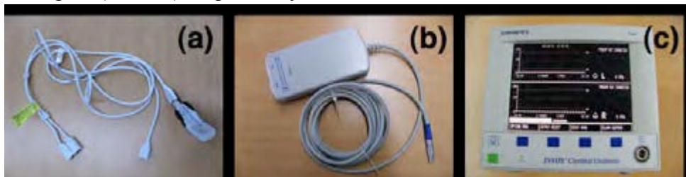
Fig. 4 : (a) A SomaSensor for performing cerebral oximetry on patient's forehead, (b) its amplifier module and (c) INVOS 4100 station.
