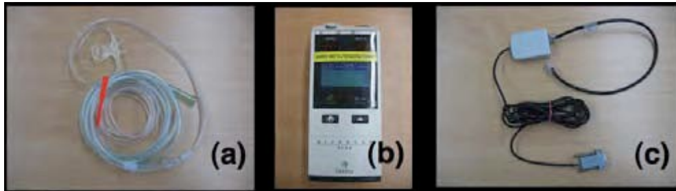
Fig. 3 : (a) Patient's EtCO 2 pipe, (b) Microcap Plus and (c) a communication adaptor kit.
