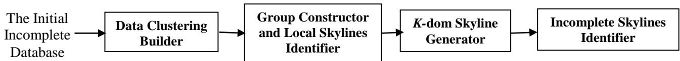
Fig. 2. The proposed model for processing skyline queries in a database with missing data
