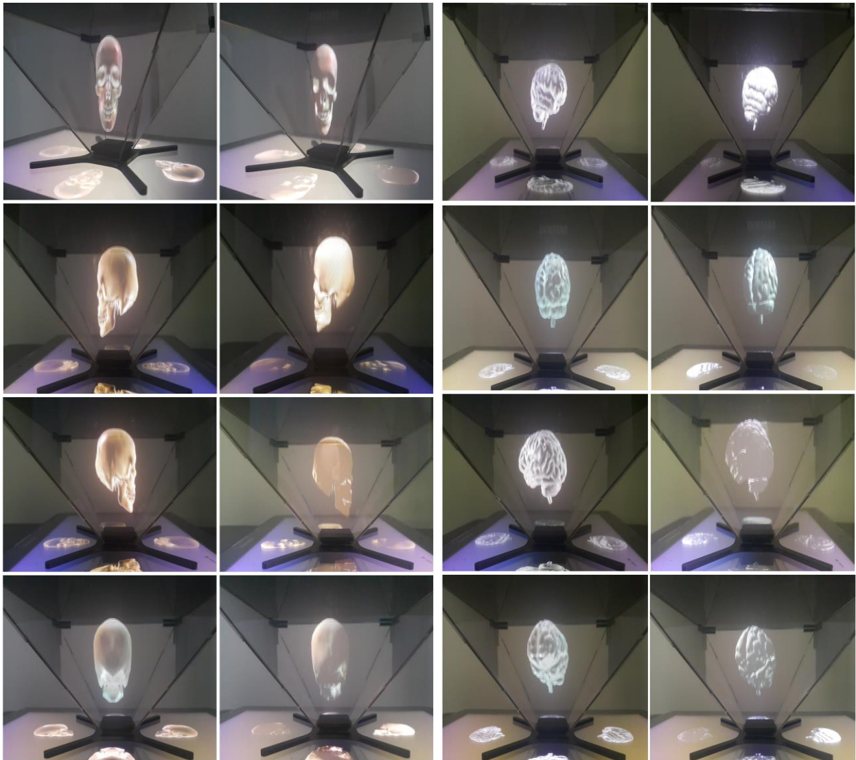
Fig. 8. The medical object inside the hologram pyramid display from the left lighting hologram style and from the right traditional lighting style
