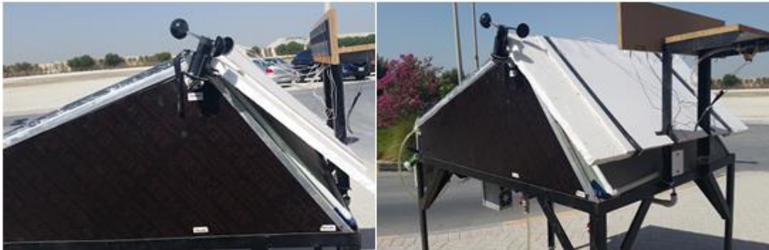
Fig.4. Styrofoam board protecting the condenser from direct sun rays.
