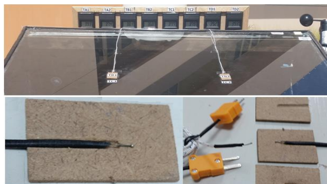
Fig.5. Thermocouple fixing arrangements.
