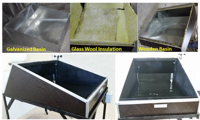
Fig.2. Solar still with built-in condenser major parts
