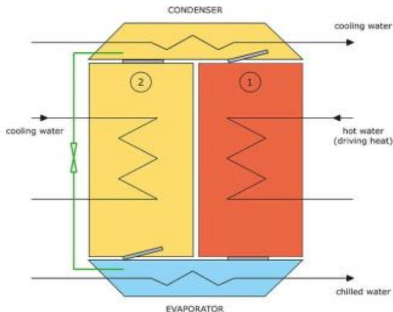
Fig.4. Schematic drawing of an adsorption chiller (SOLAIR)
