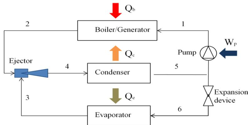
Fig.8. Schematic diagram of Ejector refrigeration system
