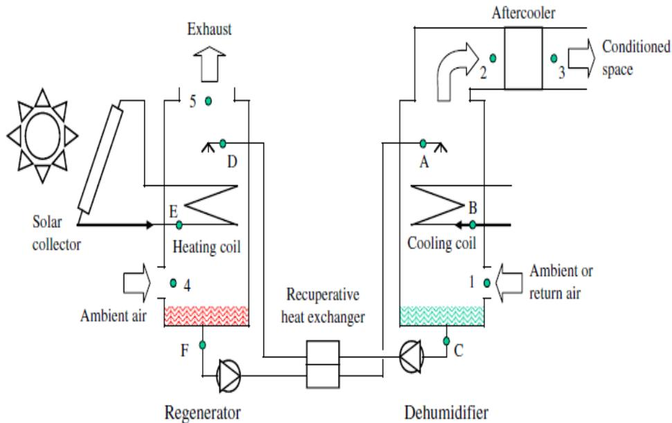
Fig.7. Liquid desiccant cooling system with solar collector (Kim & Ferreira, 2008)
