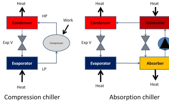
Fig.2. Main components of the absorption chillers compared to compression chillers.
