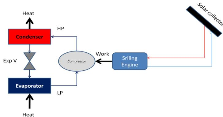
Fig.10. Schematic drawing of the solar thermal cooling system with Stirling engine.
