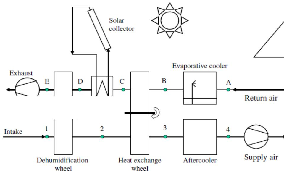
Fig.6. A solid desiccant cooling system with solar collector (Kim and Ferreira, 2008)
