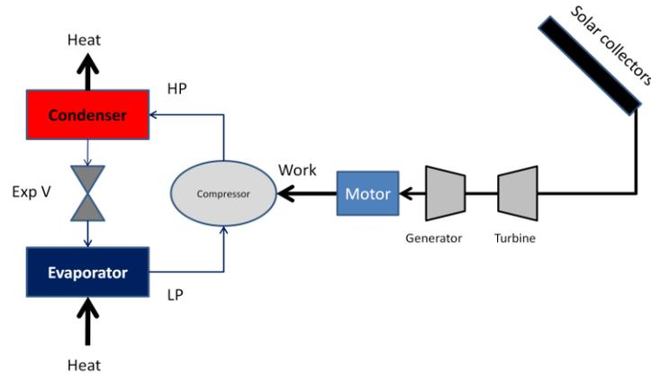
Fig.9. Schematic drawing of the solar thermal cooling system with turbine and generator.
