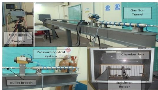
Fig. 4. Gas gun tunnel to test the specimens
