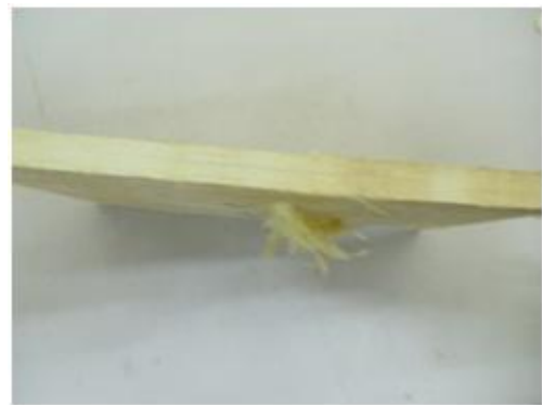
Fig.16. The damage occurred of tip nose Steel4340 bullet at 320m/s velocity on 12mm thickness of target.
