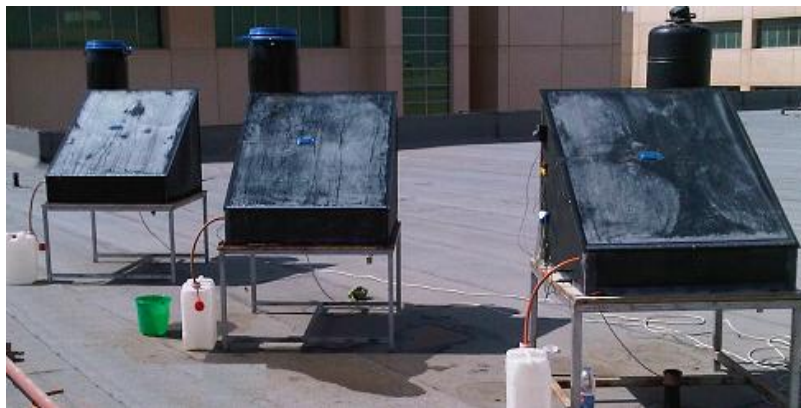
Fig.6. the three solar stills set up in situ.
