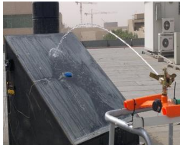
Fig. 4. Water sprinkler system
