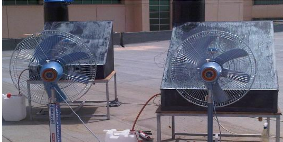
Fig.5. Fans used to vary and control wind speed
