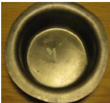
Fig. 7 (a) Perfect cup in experimental test
