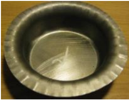
Fig. 5 (a) wrinkling in experimental test
