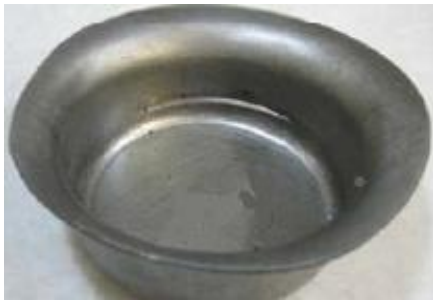
Fig. 6 (a) Tearing in Experimental test
