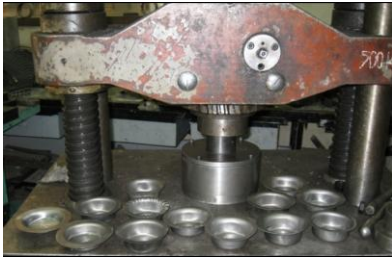
Fig. 2 Produced cups and the hydraulic press
