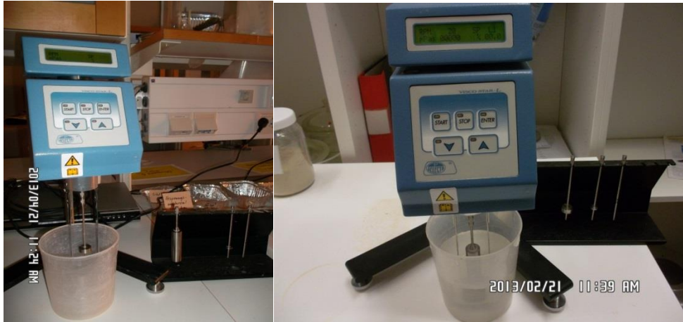
Fig. 3. Rotary Viscometer with Coaxial-cylinder spindle
