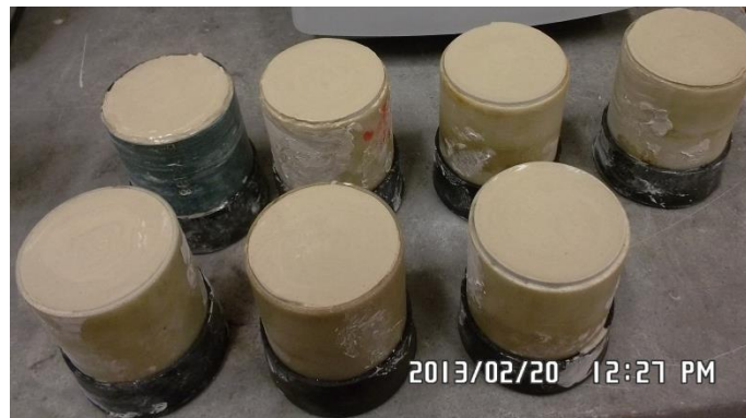
Fig. 2. Grout samples prepared for compressive strength test.
