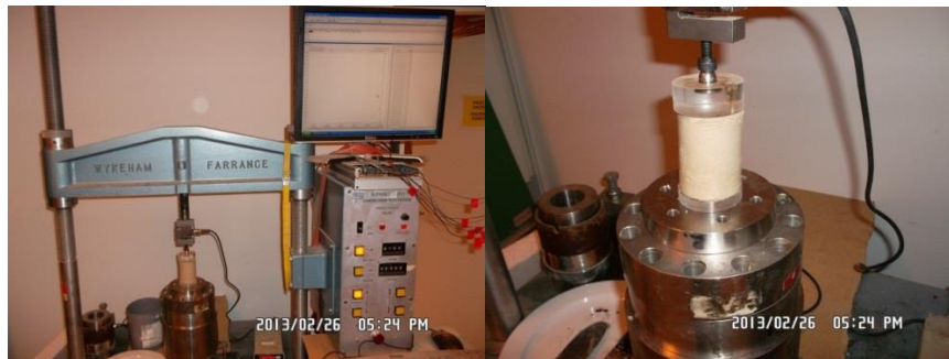
Fig. 5. Compressive strength machine used in this study
