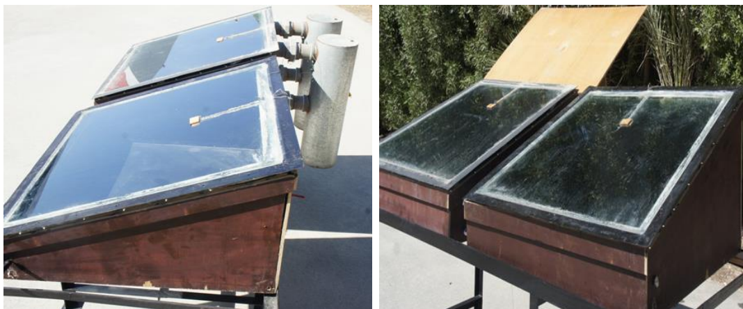
Fig.3 The two solar stills in Situ
