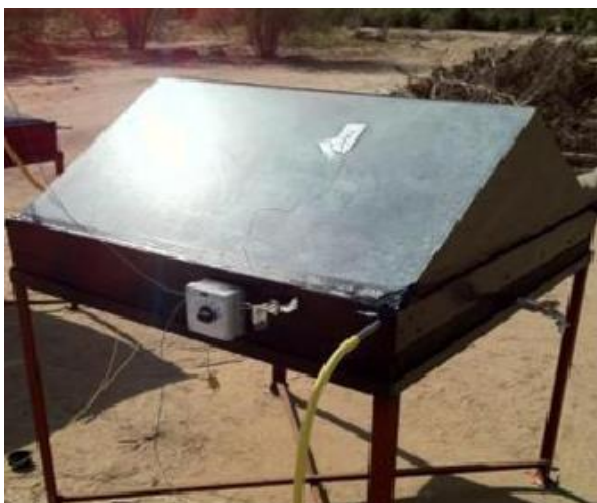
Fig.4. Double Slope Cover Arrangements.
