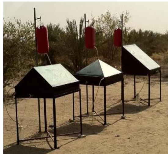
Fig.7. The three stills configurations in situ
